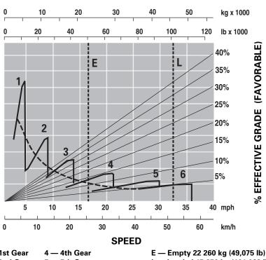
1 — 1st Gear 2 - 2nd Gear 5 — 5th Gear 3 — 3rd Gear 6 - 6th Gear
