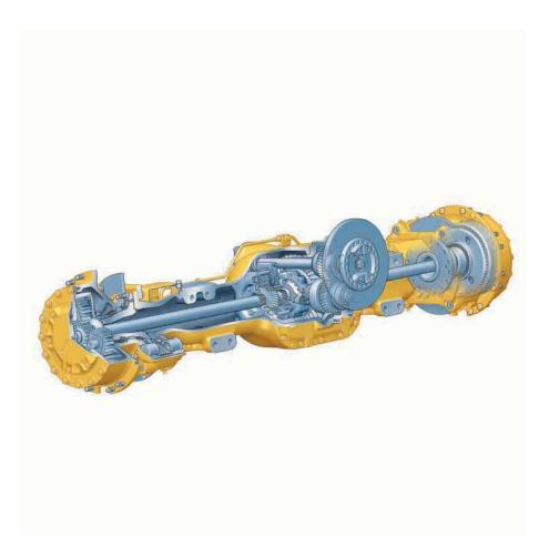
**Front Suspension.** The three-point front suspension oscillates  $\pm 6^{\circ}$  to provide a smooth ride, allowing the 725 to travel at speed over rough terrain and softening impact loads on structures and components.
