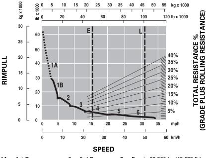
1A — 1st Gear 3 — 3rd Gear (Converter Drive) 4 — 4th Gear 1st Gear 5 — 5th Gear (Direct Drive) 6 - 6th Gear
