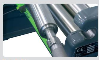
**Pivoting Top Roll** Pivoting top roll for easy removal of finished workpieces.
