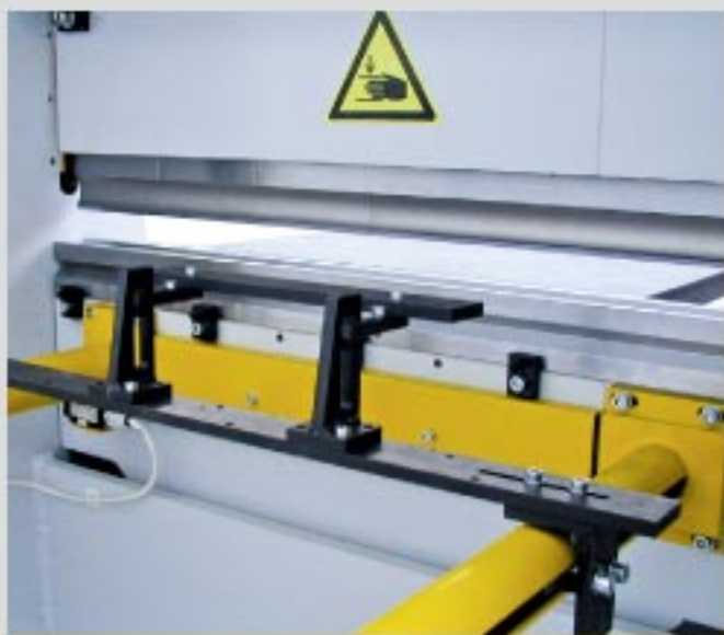
Electric back stop – to be operated in front
