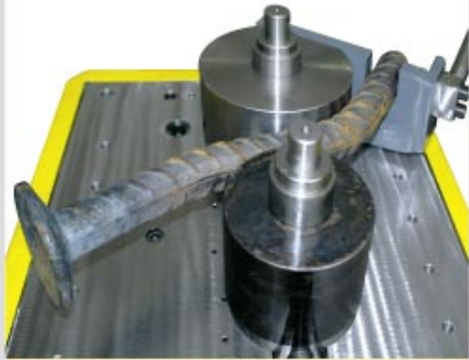
Bending of round material 40 mm
