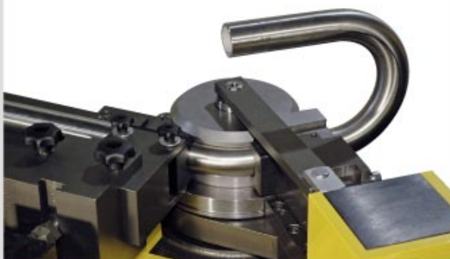
Bending head with slide bar, clamping jaws, bending form and tube d = 42 mm
