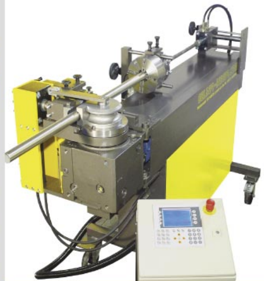
Mandrel bending machine type S-50 with 2 m length over mandrel
