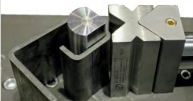
Tight bending (50 x 50 mm) around the mandrel
