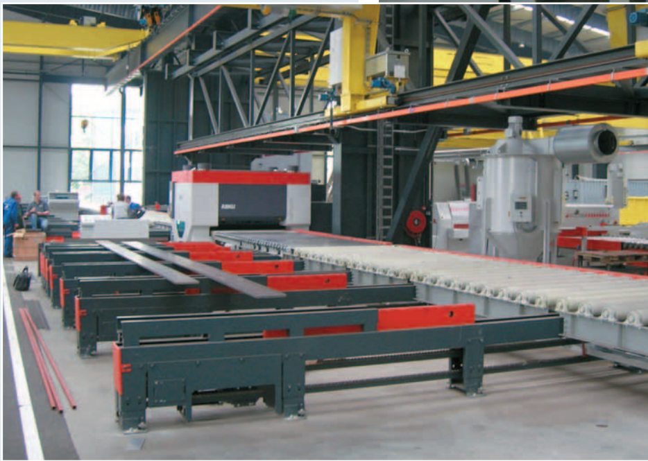
New production hall – via roller conveyor the FlatMaster® 120 is integrated in the cutting line.
