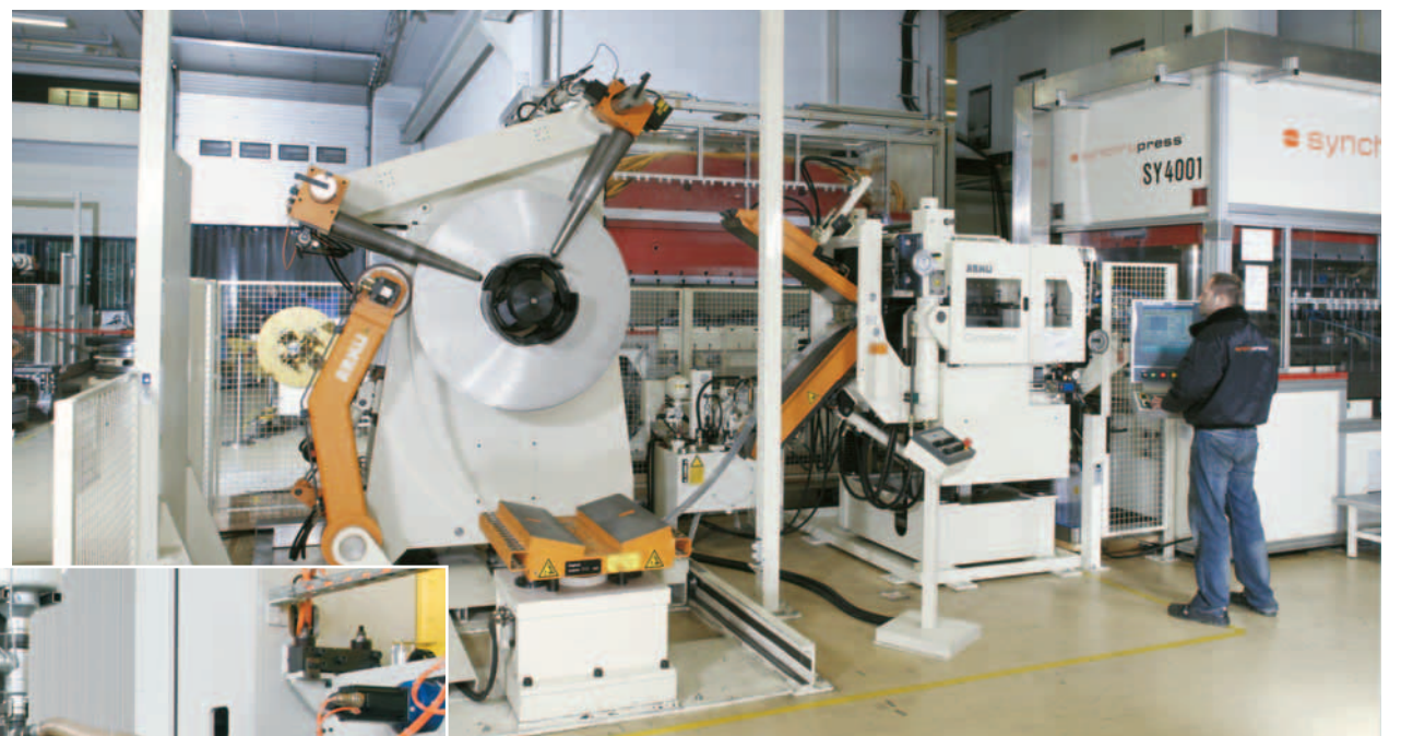
An ARKU CompactFeed® coil line with a 400t SynchroPress at Härter Stanztechnik in Germany. ( www.härter.com )
