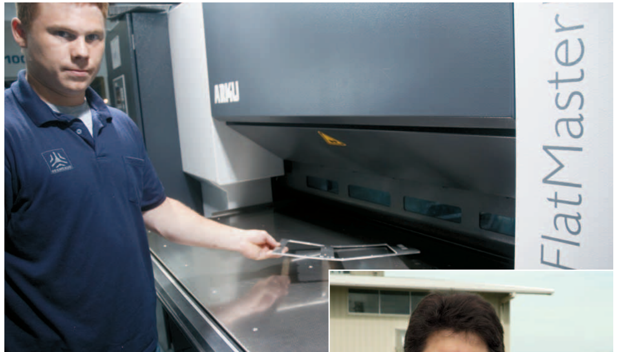
BEGNEAUD Manufacturing-employee, leveling parts with the FlatMaster® 50
