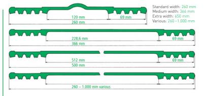
joint connections at branches in accessible pipes or as an end seal for liners.
