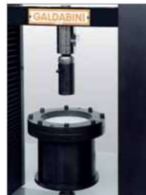
Perforation test on a geo-textile material
