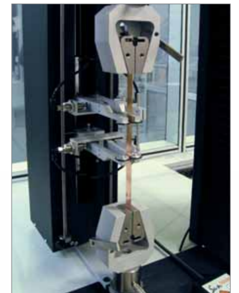
Manual wedge grips of 5kN capacity for sheet materials and other rigid samples.
