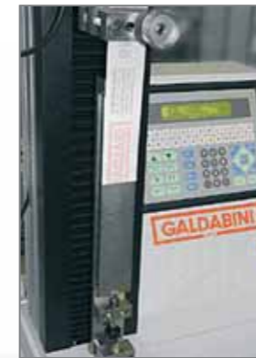
180° peel test typically used for testing adhesives.
