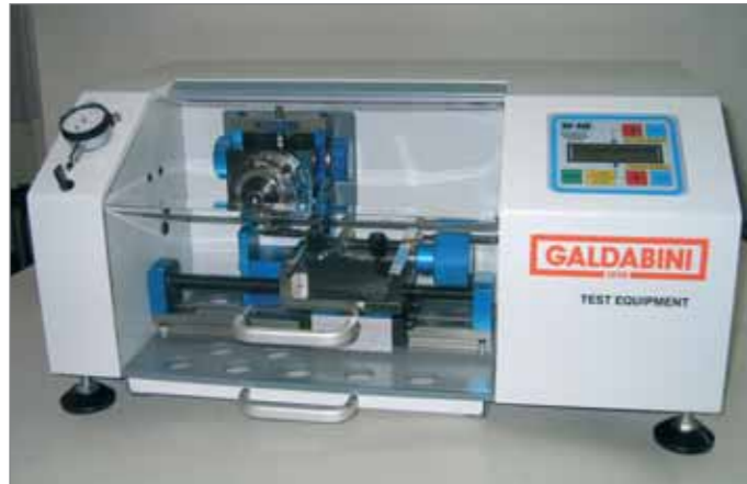
This automatic test sample notch cutter can be set to precise notch depths for Izod and Charpy samples according to international standards.
