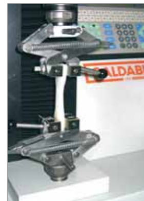
Self tightening scissor grip for polyethylene, rigid and semi-rigid materials.
