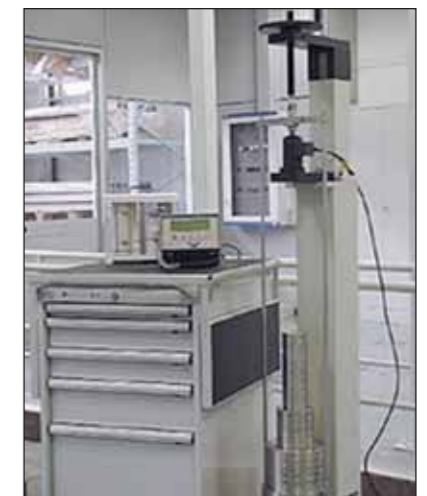
Dead weight calibration station up to 2.5 kN
