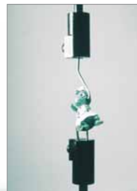
Tensile test on toys to verify product safety.
