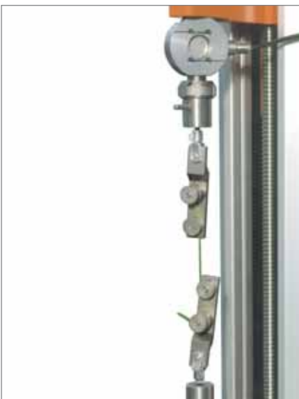
Tensile tests on fine wires can be done with this auto centering bollard grip.
