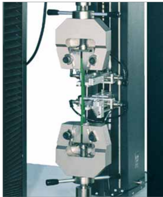
Extensometer PLAST used for high elongation measurements up to specimen failure.
