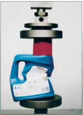
Compression test on a manufactured product.
