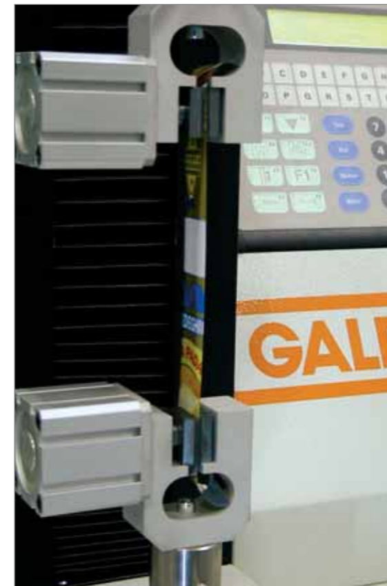
Pneumatic grips testing a 30mm wide film sample.
