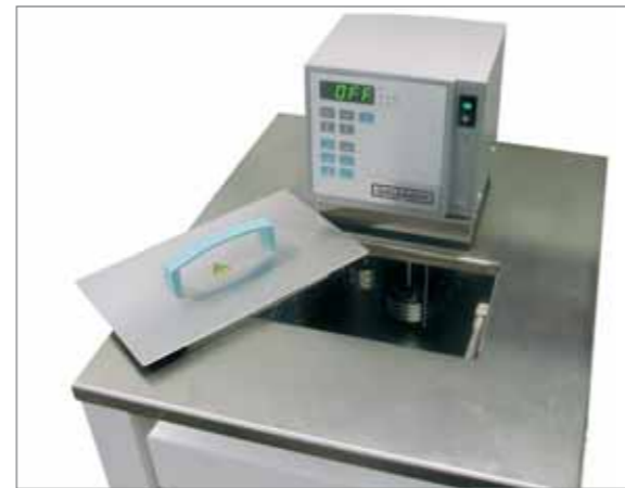
Automatic cryogenic system to condition test samples over the range -50°C to +200°C.
