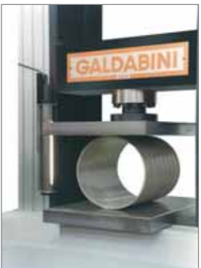
A compression tests on rigid plastic pipe section to determine radial loads.
