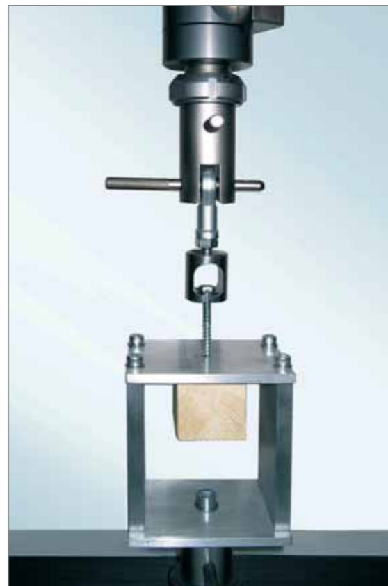
Screw extraction from a wood block.
