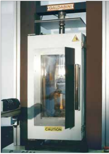
Chamber being used with optical extensometer.
