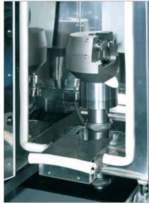
Removable panels allow the chamber to be moved without having to take off the test fixtures.
