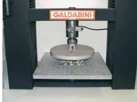
Compression test on expanded foam according to ASTM with holes for air exhaust.
