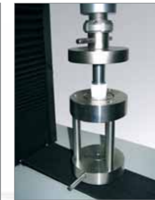
Dilation test on plastic tubes.
