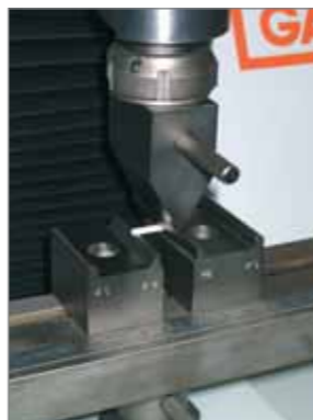
Three point bending test on a small sample. Specific fixtures for composite and ceramic materials are available.
