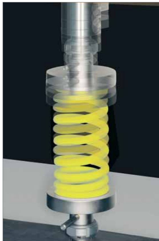
A cyclic test on a plastic spring used with our specific software application.
