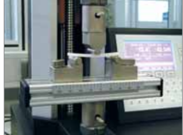
Standard 3 point bend fixture used on a single column machine.
