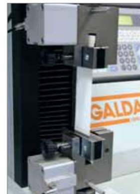
Pneumatic grips used for tensile tests on wide textile or non-textile samples. Shown with a 100mm wide sample.
