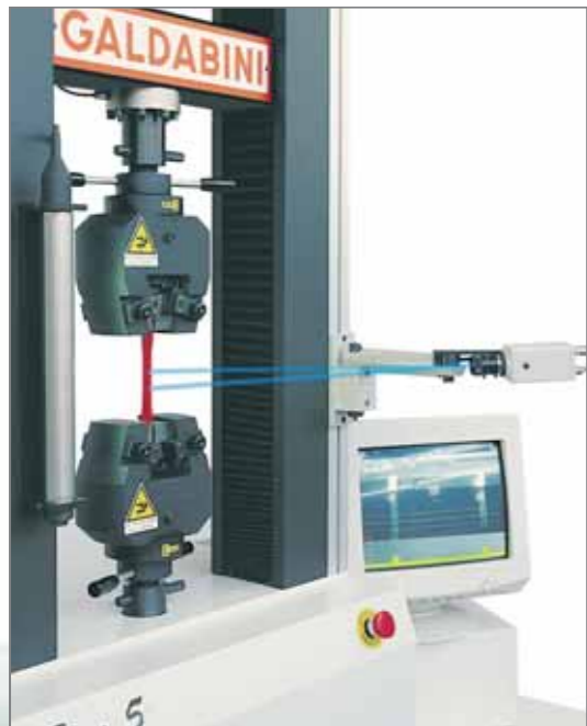
Universal Optical Extensometer with camera for tensile, compression, and flexure tests on specimens and manufactured products which can also be used in an environmental chamber.
