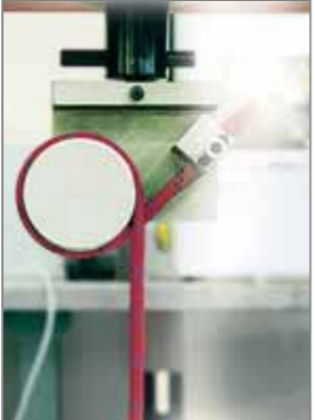
A bollard type grip used for tensile testing cord.
