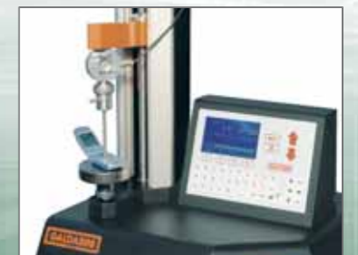
Cyclic compression tests on a cell phone keyboard.
