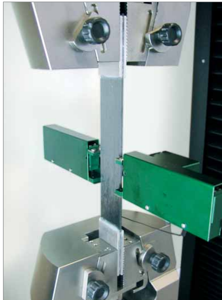
Extensometer STRAIN-BIAXIAL for composite materials is used to measure longitudinal deformation and to determine Poisson's ratio.
