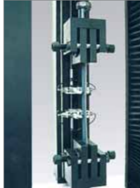
Special grip used for a tensile test on conveyor belt material
