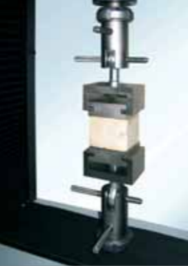
This grip is used for measuring the pull apart forces on a glued wood block.
