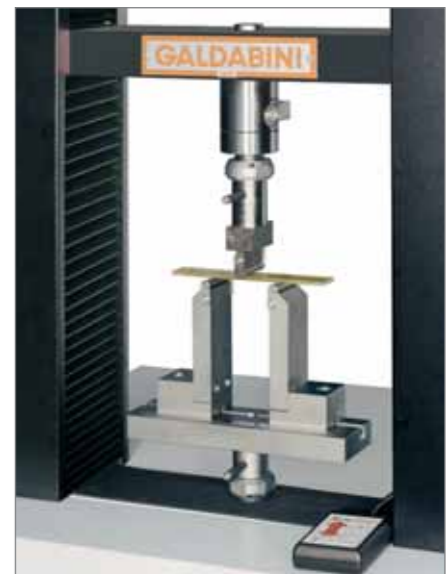
A 3 point bend fixture suitable for use in an environmental chamber. Many versions are available with variable span, and interchangeable supports. These meet international standards such as ASTM and ISO and can be used in an environmental chamber and fitted with precision transducers to measure flexural modulus.
