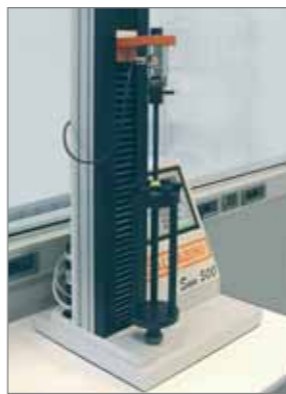
Penetration test on plastic film.
