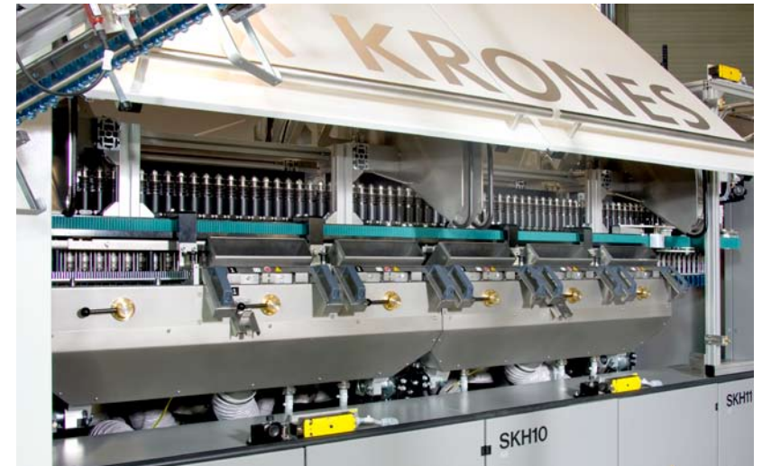
Perfect access to all areas of the heating module
