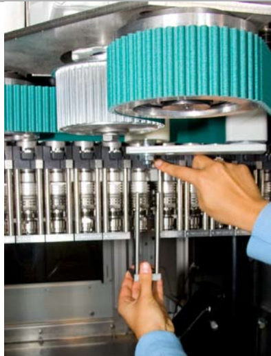
Product change-over on the heating module
