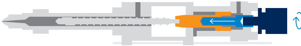
Linear force transmission ensures maximum shot weight constancy
