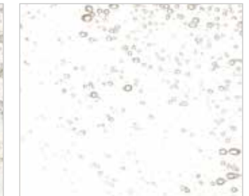
polyalphaolefin (PAO) air release: 12 seconds
