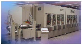
The pressure controlled grinding combined with grinding to size for screwed cylinders of up to 16m length reduce a 2 step operation to one single pass operation in a single machine. Tremendous production increase with reduced handling is the result.
