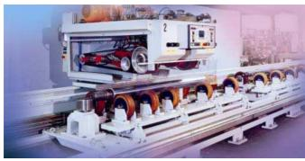
The same technical principle for high speed grinding instead of fine turning has now been developed for Company VSMPO-AVI SMA/Russia for improving of Ti billets surface up to Ø 450 mm.
