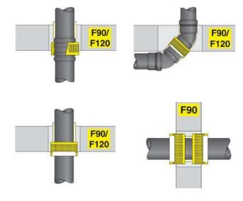
Pipes guided through ceilings or walls must be absolutely fire- and flue gas-proof for a minimum period of 90 minutes in case of fire. The extremely flat FRIAPHON fire-stop collars – even approved for direct installation on sockets – meet this requirement.
