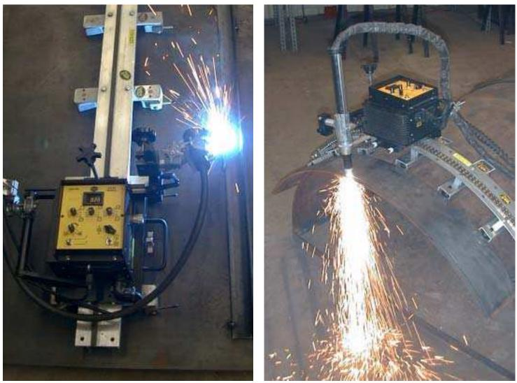
The modular design allows the user to quickly reconfigure the unit for straight line cutting or welding, stitch welding or weave welding, all with the same machine!
