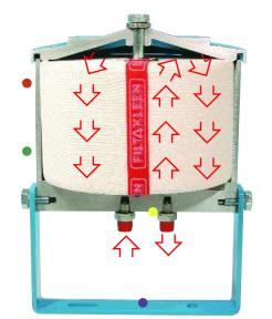
The high tech cartridge gives continuous all round protection against water and ultra-fine debris with contaminated oil entering the filtakleen unit at the base flowing up the centre tube through the 1 micron filter before flowing back to the hydraulic circuit. Flow rates through filter 4.1 l/min to 6.1 l/min depending on unit fitted.
