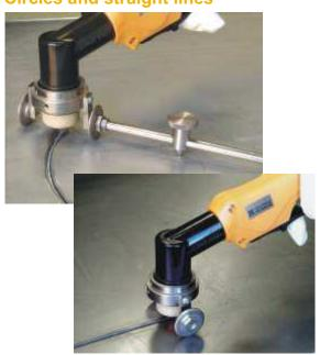
Guide wheels with circle attachment for circle cutting as well as for straight line cutting along markings
