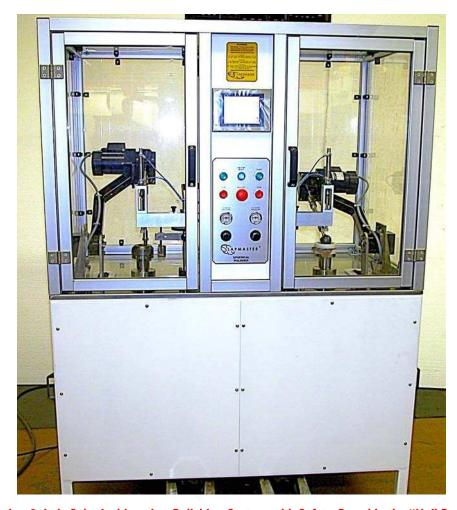
2-Station 3-Axis Spherical Lapping-Polishing System with Safety Guard in the "Up" Position
