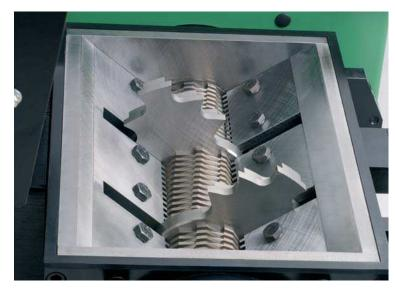
The crusher blades break down plastic waste to a size that feeds into the teeth of the cutter wheels. Broken waste is continuously swept back into the cutterhouse chamber by the blades as they rotate.
