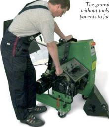
As waste feeds into the cutting wheels, the teeth cut the pieces cleanly into high-quality granules of uniform size. The reinforced teeth and powerful slowspeed cutting action easily slice through the hardest materials.
