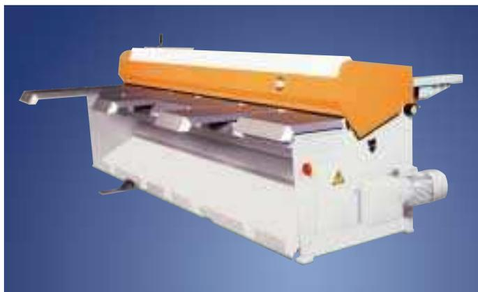
■ The SMARTcut swing beam shear positions the part either with a powered backstop or with the front operated manual backstop. The standard configuration also includes a sheet support system and a part sorting
