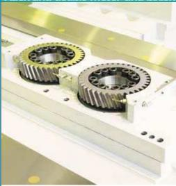
The use of a Rack and double motor and pinion to drive the X and Y axes (longitudinal and cross, respectively) is one of the main traits common to most of the machines that ZAYER manufactures.
