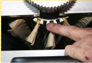
Additional cleaning brush for the vacuum transport belt
