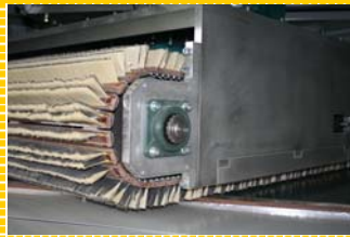
Brush belt for a gentle surface sanding in all areas
