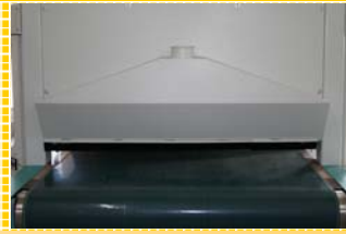
Special vacuum transport belt for save work piece transport
