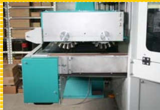
Double brush aggregate at the run out of the machine
