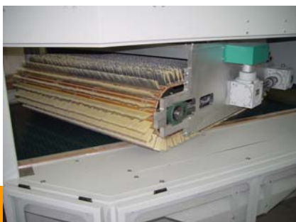
The Roba Tech sanding belt contains 174 abrasive segments
