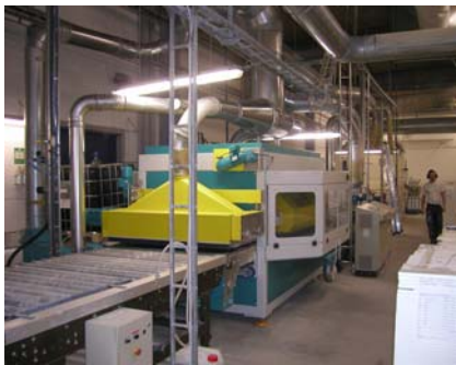
Roba Tech integrated into a furniture production spraying line
