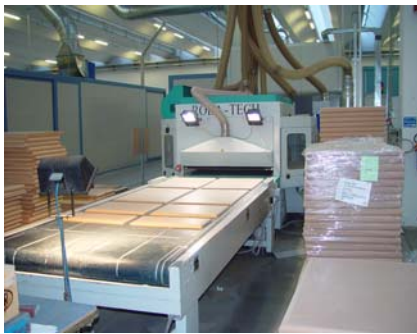
Roba Tech integrated into a cabinet door membrane press production line
