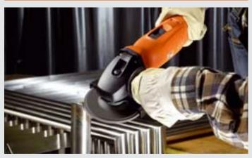
The adjustable speed range of 2500/min – 7000/min makes the WSG 14-70 E a universal angle grinder (for machining stainless steel for example).
