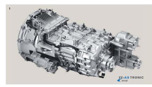
■ Gentle gear changes protect both the clutch and the downstream driveline. If the driver wants to get involved and change gears manually, he or she can use the push-button switch. It applies for both the automatic and the manual mode: Incorrect shifting excluded thanks to the electronic control unit.
