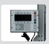
The program consists of sections, where each section is provided with a bending value. This enables easy and quick programming of the machine for different bending operations. The CNC system can operate with "interpolation", where the rolls are adjusted simultaneously with the feeding operation.
