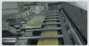
The unit consists of a driven roller way and a pneumatic pushing device for punching the blanks (Alu-sheets) into the roller. The concept makes it possible to integrate a punching line with Luna 8835/8344. Unit 1700 is equipped with a slave computer connected to the control system of the bending roll. The unit can be installed or removed in about 5 min.
