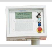
The programming of the machine is facilitated by different menus available on the screen. In order to further simplify the programming, the control buttons are of multi-function type, whose functions are automatically changed when changing menus. The CNC has a storage capacity of 200 programs with 50 lines in each
