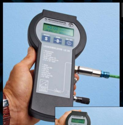
Handy with high pressure: leak simulator LS 26
