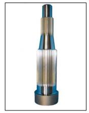
C45 bar stock 100 cm in diameter was machined at a cutting rate of 90 m/min, and two types of shaft with differing parameters were produced: one 50 mm in diameter with 23 teeth, machined at a speed of 1035 min<sup>-1</sup>, and a second, 80 mm in diameter with 39 teeth and machined at a speed of 1026 min<sup>-1</sup>. The feed was 1 mm in each case, with a cutting depth of 4 mm. *The tool's gear ratio is* 3:1 (Fig. 2).
