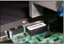
pecialty Tamp Alternativ For situations where very small labels need to be applied, such as circuit board applications, the PA1200 supports custom Tamp sizes, which will permit labels as small as .20" wide x .20" high.
