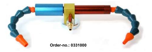
The *ARIANA* Hot & Cold-Gun is driven by compressed air and is used for punctual heating or cooling of metal and plastic parts on machine tools. It features a dual function: producing both hot and cold air. The hot air is used for fast drying and heat treating. The cold air is especially used where the application of coolants and lubricants is not desired. The Hot & Cold-Gun is also used in laboratories for several applications.
