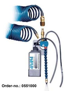
The *ARIANA*-Micro-System is based on a coaxial spray nozzle, which generates a round stream. By means of turning the spray nozzle, several spray cones can be generated for many applications. The coaxial sprayer works pneumatic and is provided with a medium by a separate unpressurized container.
