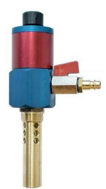
The *ARIANA*-Power-Vac-Pump is a dual acting suctionforce pump operating with compressed air. It is mainly used for the filling and deflation of coolant and lubricant containers. The tool is designed for a fast and smooth installation on a barrel. It is screwed on the barrel's faucet hole (3/4 inch) and connected with compressed air. A conveyer tube is mounted on the other barrel's faucet hole (2 inch).
