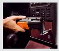
With the MINICUT and File Set even the tiniest of cuts <sup>3</sup>/<sub>8</sub>" and above are not a problem, even in difficult-to-reach places. Available for plastics, metals and wood.
