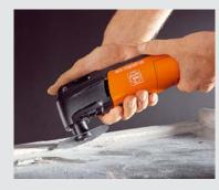
Brittle puttied edges can be removed without any problem and without any danger of glass breakage.
