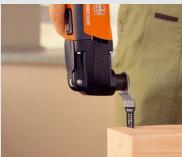
Saw into wood 2 %" deep with the new universal E-CUT saw blades.
