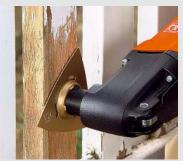
With the carbide rasp, remove stubborn signs of weathering thoroughly and quickly thanks to the high sanding capacity.
