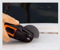
The round HSS saw blades are excellent for sawing work on fibreglass and carbon fiberglass reinforced plastic hulls. Make perfectly clean cuts (0.5 mm wide) without any cracking or damage to the laminate.
