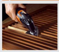
The flat sanding pad also gives access to tight spaces, e.g. the slats of shutters.
