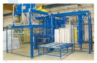
Picture 1 – HEITZ HBB 1412: Moulding machine with handling robot and stacking table. For the production of ICF elements with sheet metal or plastic connecting inserts, 3 elements per cycle.
