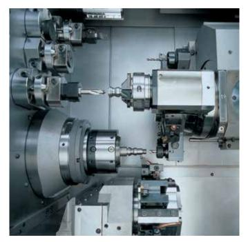
The INDEX ABC has 2 tool turrets with 14 tool mountings. An upper turret with 7 tool stations plus a fixed station for mounting a synchronous spindle (for chuck or collet clamping) and a lower turret with additional 6 tool mountings. Plus five back-boring stations (of which 2 are live) for cutoff-end machining. Optional polygon turning unit
